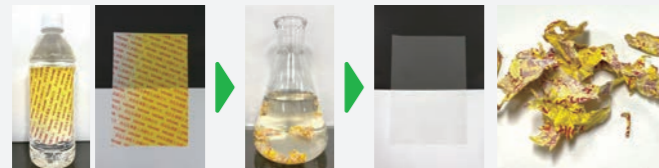
After stirring in an alkaline solution of 80°C, 1.5wt% (concentration) sodium hydroxide for 10 minutes, rinse with water.
